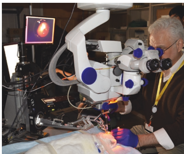
Fig. 3 The Steady-Hand Eye Robot developed by Johns Hopkins University
